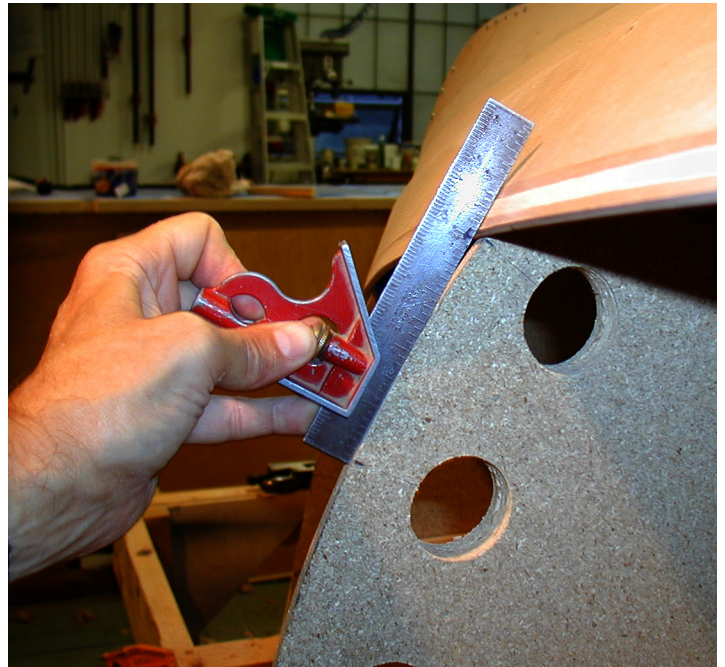
Each lap is beveled and checked against the mold with a straight edge to the line indicating the top edge of the next plank.
