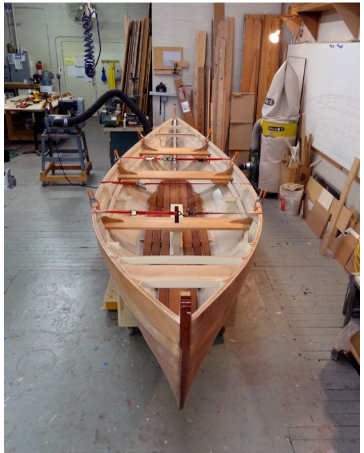
Ready for side benches.
