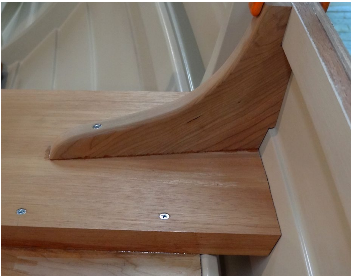
A finished knee. The small gaps will close up when the knee is fastened in.
